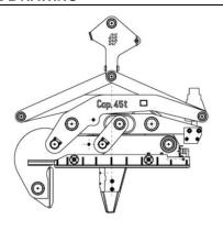
Heppenstall vertical coil tongs are designed to accommodate custom coils of all dimensions.
